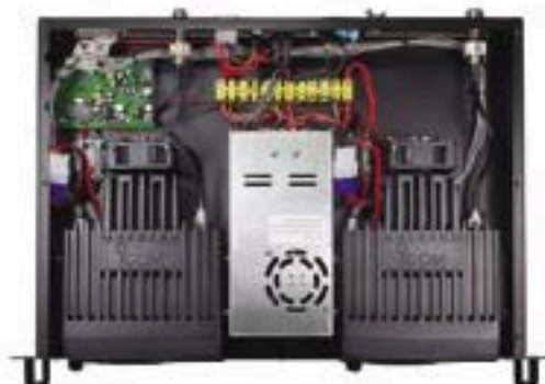
Radios, controller, and power supply, all in one box. Dual broad-air fans keep the unit cool. 19" Rack mountable. Battery backup capable.
